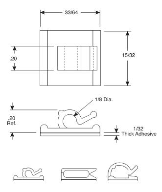
EPD Adhesive backed nylon wire and cable clips are used to route wires and cables.
